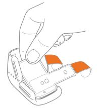
3. Press down to secure the sensor. The sensor should sit flush in the boot.
